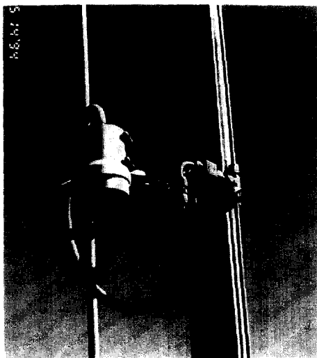
Fig. 1. Photograph showing a MT and a PUF sampler mounted at the 150-cm height on the sampling mast.
